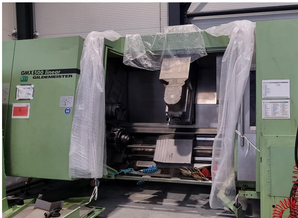
CNC turning- and milling center with main and counter spindle for efficient 4-axis complete machining of chuck, bar or shaft parts
